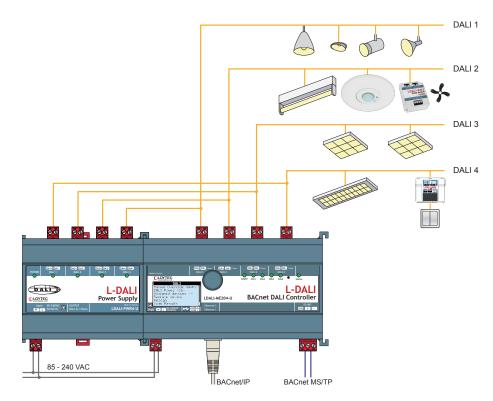
L-DALI Controllers are multi-functional devices featuring DALI light control and gateway functionality between the DALI protocol (Digital Addressable Lighting Interface) and LonMark Systems or BACnet Networks. In addition to the integration of DALI ballasts these controllers support configuration of DALI pushbutton couplers (e.g. LDALI-BM2), a variety of multi sensors (like the LDALI-MS2), and the L-DALI relay modules (LDALI-RM3 and LDALI-RM4).
