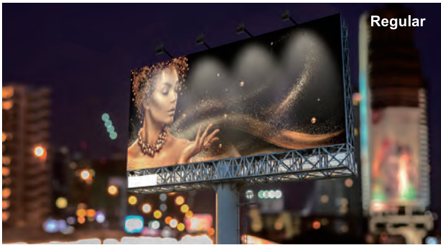
Low uniformity and obvious dark zones, and the central illuminance is high.
