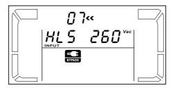
Parameter 2 & 3: Set the acceptable high voltage point and acceptable low voltage point for bypass mode by pressing the Down key or Up key.
